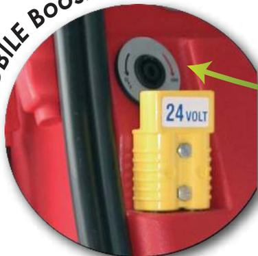
Male 4 pole plug to connect to the charging plug on the front of your MOBILE Booster Unit
