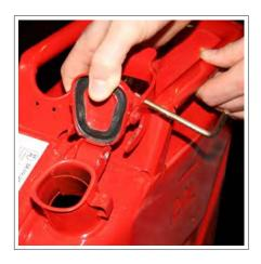
4. Place your thumb on the very front of the lid lip and push towards the back of the can. This should bend the date stamped plate until it is straight again.
