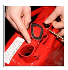
3. To repair a bent lid, open the lid out until it sits in the 'open-locked (down)' position as per image.
