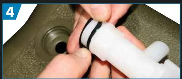
Wrap seal back into position, noting the blue marker edge remains facing away from tap thread.
