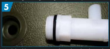
Seal should now taper towards tap thread, reducing the area of contact it makes with can thread when tightened.
