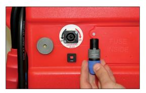
Insert the charging plug tester into the female charging plug, and turn to the right (as per the red arrow), to turn it on.
