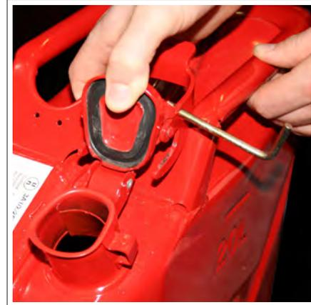
4. Place your thumb on the very front of the lid lip and push towards the back of the can. This should bend the date stamped plate until it is straight again. If this does not quite get the plate flat, you can use a piece of plywood to assist.
