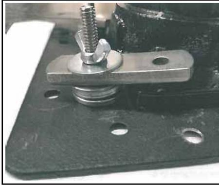
Add 1 or 2 washers on top of the clamping tabs and tighten down the wing nuts onto the tabs, until you feel that your Bottle Jack is securely attached to the Base Plate Insert.
