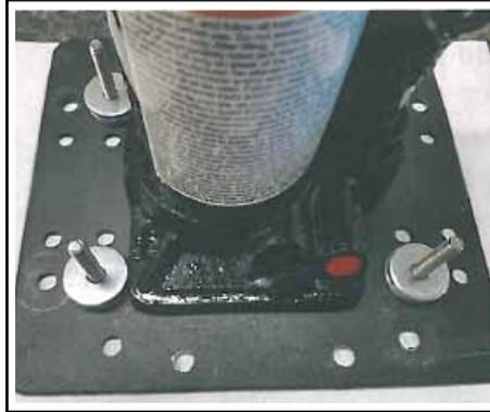
Set your bottle jack on top of the base plate in the middle of the screws as shown. Screws can be moved to accommodate various sized jacks, so spend some time figuring out where the screws and tabs need to be attached to the plate.
