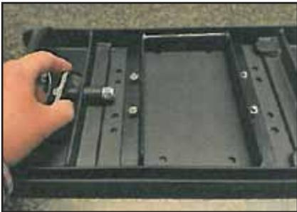
2. Pull back Quick Release Pin on Universal Base Plate to set Insert snugly, then release pin.
