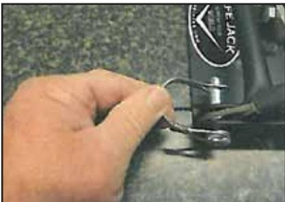
4. Secure cables with Clevis pins.
