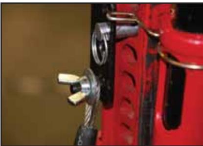
8. Cables may be tightened or loosened somewhat by adjusting the wing nuts on each side of the upper clevis. Adjust the wing nuts until the slack has just come out of the cables, with the jack foot plate resting flat against the base place Insert.
