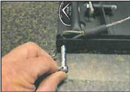
3. Attach cables to the Universal Base Plate with screw as shown.
