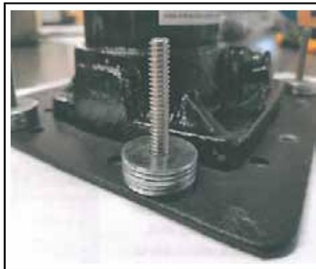
Stack washers on screws until each stack of washers is slightly shorter than the base of the jack.
