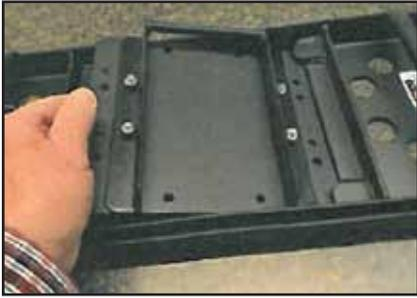
1. Insert plate with Hi-Lift shoe into Universal Base Plate, with bar of shoe on opposite side to cable attachment holes in Universal Base Plate.
