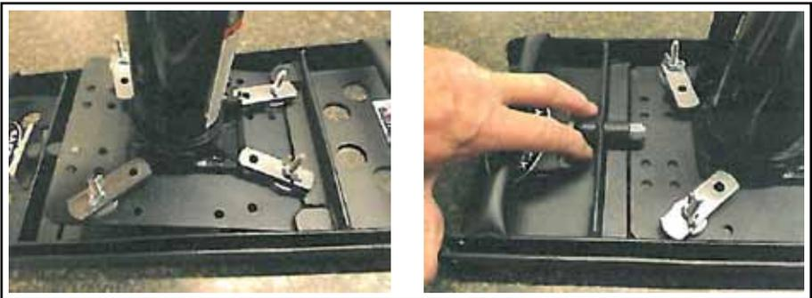
Slide one end of the Insert Plate under the two tabs on the Universal Base Plate.
