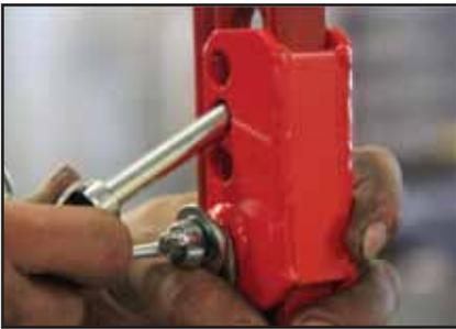
7. Pull cables up in front of the jack and pin upper clevis assembly to the front side of the jack using the Quick release pin. Ensure that you attach pin in the hole that makes the cables as tight as possible. The pin can be used to pry the clevis up to tighten the cables. Make sure the cables are not twisted and the adjusting wing nuts are at the bottom of the clevis.
