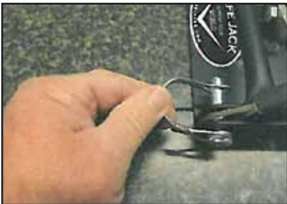
4. Secure cables with Clevis pins.
